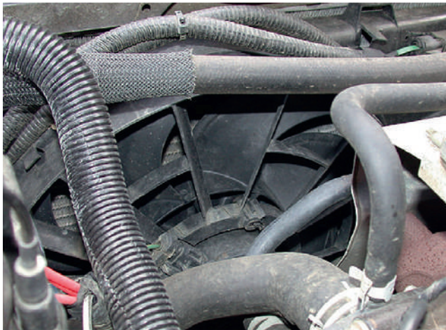
Figure 3.163 Condenser cooling fan
